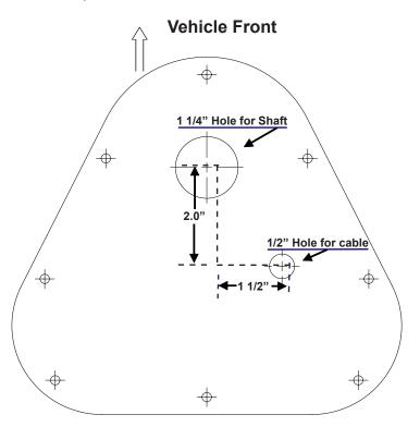
Step 2: Route the coaxial cable through the Base Assembly. Caulk the bottom of the Base Assembly with a liberal amount of non-hardening sealing compound, then position and attach it to the roof with eight #8x1" pan head sheet metal screws. Seal the edges of the Base Assembly and the top of the screws with sealing compound.
